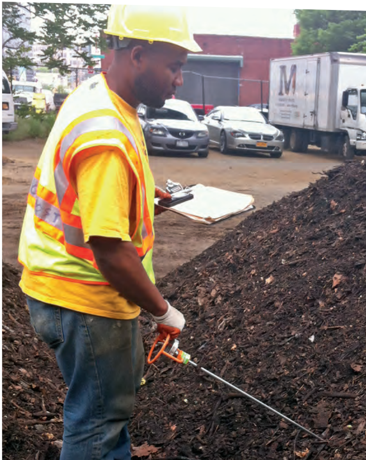
NYC Master Composter Chris Bivens monitors the temperature of a windrow.
