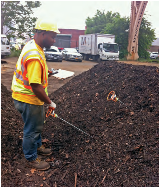
To use a compost thermometer, simply push its metal pole into the center of your compost and read its temperature.
