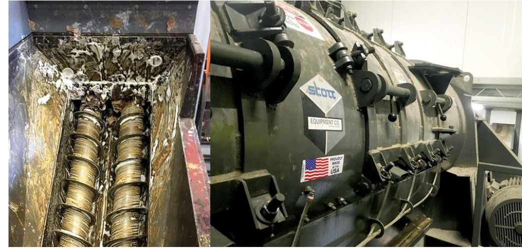
Twin screws in the bottom of the feed hopper (left) tear open cardboard boxes and other containers while conveying the contents to the separator.
